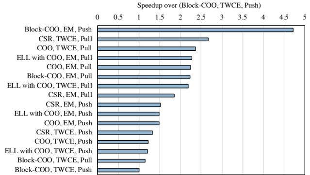
**Figure 10: Performance comparison among different tuning options for PR with LJ. Four topology layouts (COO, CSR, ELL+COO, Block-COO), two schedules (EM, TWCE), and two directions (Push, Pull) are compared. The baseline tuning option is (Block-COO, TWCE, Push).**
