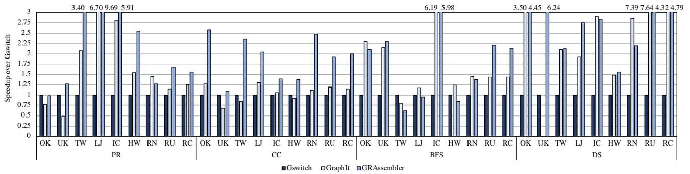
**Figure 8: Performance comparison with the state-of-the-art graph processing frameworks such as GraphIt and Gswitch. Each graph shows speedups over Gswitch. Four algorithms on nine graphs are used on NVIDIA GeForce RTX 3090 GPU.**
