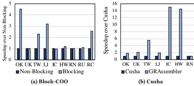
**Figure 9: Extending topology layout library. (a) shows speedup of Block-COO over COO using GRAssembler interface. (b) shows speedup of GShard topology layout over original GShard implementation of Cusha [16].**
